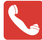
Emergency Fire Telephone
